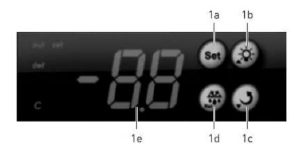
1a. Temperature adjustment button, press and hold for 3 to 4 seconds until the indication "St" appears to enter the adjustment mode. Press the button again to adjust the temperature of the device. After 30 seconds of inaction, the new set temperature is automatically saved.
