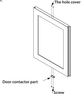
**6.**Hold the Door carefully with your assistant and place it on the top of Bottom Hinge, make sure the Pivot Hinge is at correct place through the Hinge Washer. Insert the pin of the Upper Hinge into the Bushing on the top right and fix it with Hex Head Screw (4pcs). Cover the Upper Hinge and Bottom Hinge with Upper Hinge Cover and Bottom Hinge Cover. Cover hinge screw holes
