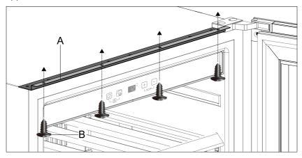
A· Top Bracket B· 4 Screws (ST4.2\*12mm)
