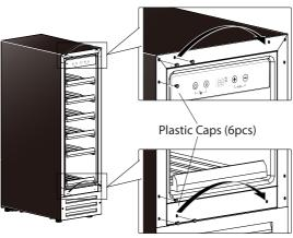
**5.**Install the Upper Left Hinge and Bottom Left Hinge to the left side of the cabinet. Make sure the screws are tightened.
