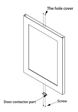
**7.** For a wine cooler without lock, please turn the door by 180° (upside down). For a wine cooler with lock, keep the door upright and remove the lock hold cover from top to bottom, then turn the door by 180° (upside down).
