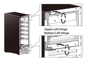
**6.** For a wine cooler with door contactor, firstly, remove the top hole cover, and remove the bottom door contactor part on the door frame
