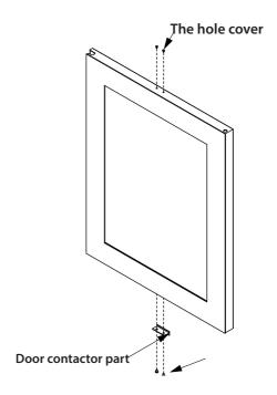
**4.** For a wine cooler without lock, please turn the door by 180° (upside down). For a wine cooler with lock, keep the door upright and remove the lock hold cover from top to bottom, then turn the door by 180° (upside down).
