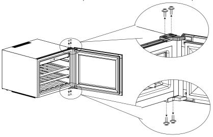
o Unscrew the 3 screws from Top Bracket, move the bracket to the right end and screw the 3 crews.
