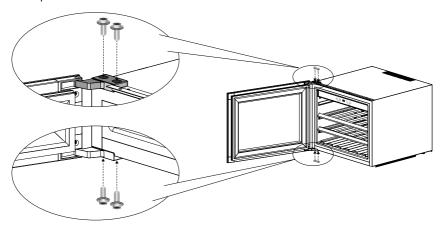
oThere is door contactor at the top and bottom door frame, when reversing the door, no need to change any door contactor parts.
