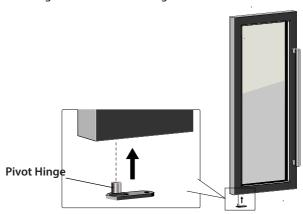
$\textbf{10}. In stall the door to the le<u>ft hinge side by tightening the Pivot Hinge with the 2 screws.}$ </u>
