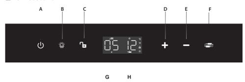
A. Power B. Lighting Lock/Unlock Temp. Plus E. Temp·Minus F. Zone Select G. Upper Zone Lower Zone D+E °C/°F Switch
