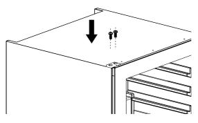
o Install the Upper Door Shaft (Left/Right) on the upper left door corner by screwing the 2 Phillips Flat Screws (M4\*8);
