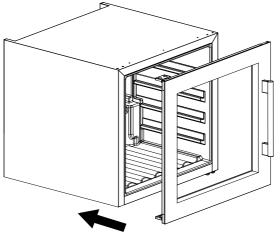
o Install the Upper Door Shaft (Left/Right) on the upper left door corner by screwing the 2 Phillips Flat Screws (M4\*8);
