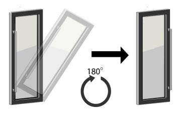
7. Insert the Pivot Hinge into the bottom hinge hole of the door.
