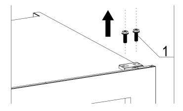
o Unscrew the 2 Phillips Flat Screws (M4\*8) from the right lower Door Hinge;
