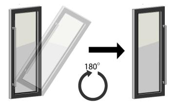
4. Hold the Door carefully with your assistant and place it on the top of Bottom Hinge, make sure the Pivot Hinge is at correct place through the Hinge Washer. Insert the pin of the Upper Hinge into the Bushing on the top right and fix it with Hex Head Screw (4pcs). Cover the Upper Hinge and Bottom Hinge with Upper Hinge Cover and Bottom Hinge Cover. Cover hinge screw holes on the top right with the Hole Cover.
