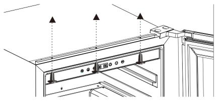
A. Top Bracket B. 4 Screws (ST4.2\*12mm)
