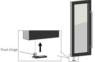
8.Install the door to the left hinge side by tightening the  $\overline{\text{Pivot Hinge with the 2 screws.}}$
