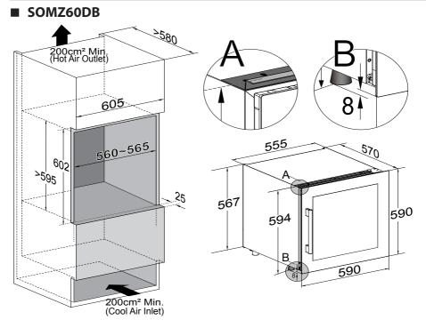
To fix the appliance with Cabinet, pls. screw the 4 screws (ST4.2\*12mm) through the Top Bracket. The Top Bracket is pre-installed on top of appliance.
