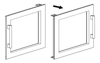
o Make sure the hole position of the left door hinge is aligned with the hole position on the cabinet;
