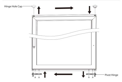
**3.**Remove the Bottom Hinge Cover by prying it off gently with small flat screwdriver. Remove the Bottom Hinge by unscrewing the Hex Head Screw (4pcs). Unscrew the Pan Head Screw (4pcs) from bottom left side. Now move the Bottom Hinge to the bottom left side and screw it tightly with the Hex Head Screws (4pcs). Move the Pan Head Screw (4pcs) to the bottom right side and screw it.
