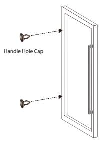
**5.**Remove the Handle Hole Cap (2pcs) on the right side of Door by prying it out gently with small flat screwdriver.
