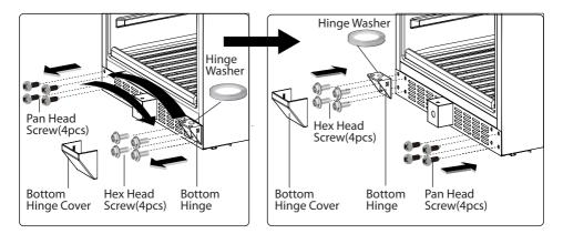
**4.**Hold the Door carefully with your assistant and place it on the top of Bottom Hinge , make sure the Pivot Hinge is at correct place through the Hinge Washer. Insert the pin of the Upper Hinge into the Bushing on the top right and fix it with Hex Head Screw (4pcs). Cover the Upper Hinge and Bottom Hinge with Upper Hinge Cover and Bottom Hinge Cover. Cover hinge screw holes
