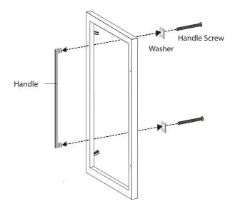
$\mathbf{7I}$ nstall the Handle to the right side of the door by screwing tightly the Handle Screws (2PCS).
