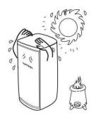
Is the location exposed to direct sunlight or too close to the furnace and other heat sources
