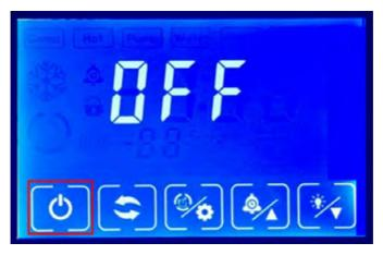
Step 3. Press **Clean/Set button**, the control panel will display clean pattern. Usually, 2 minutes to clean the machine is enough.
