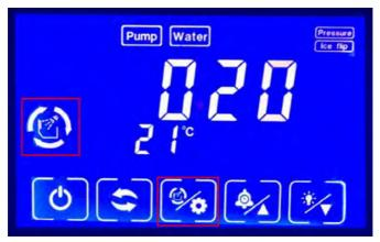
Step 4. Press Model button 3 times to back to making ice model.
