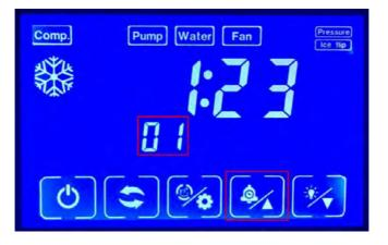
Press Light/- button for one time , the position which displays temperature will appear "-1" as the following picture. It means the ice making time will be reduced 1 min, the ice will become thin. After setting, you need no other operation, the machine will resume making ice automatically.
