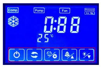
Step 2. Press Schedule/+ button, the position which displays temperature will flash "00" .
