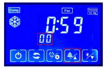
Step 3. Press Schedule/+ button and Light/- button to adjust. Press Schedule/+ button for one time , the position which displays temperature will appear "01" as the following picture. It means the ice making time will be increased 1 min, the ice will become thick.
