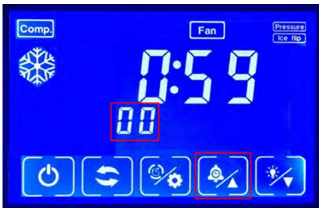
Step 3. Press Schedule/+ button and Light/- button to adjust. Press Schedule/+ button for one time , the position which displays temperature will appear "01" as the following picture. It means the ice making time will be increased 1 min, the ice will become thick.
